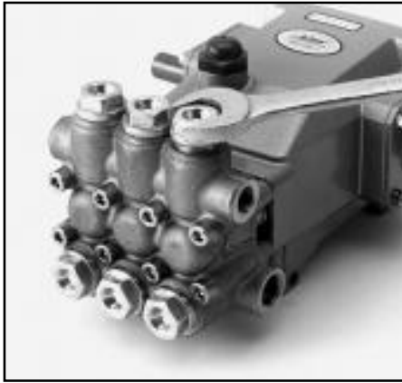
All Models Removal of Valve Plugs
